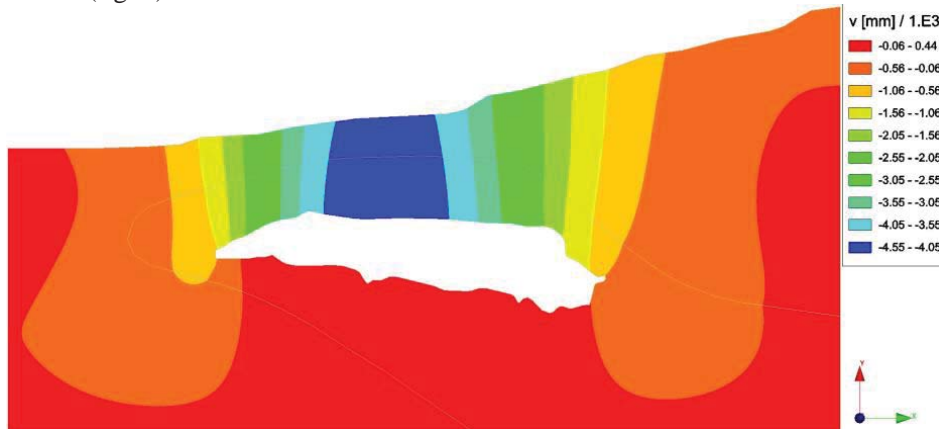
Fig. 6 Vertical displacement of the massive rocks in section 6-6` scalar representation (Option II) – v , in mm
