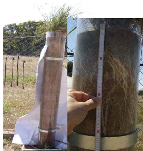
Fig. 2 Plexiglass tube for evidence of ingrowth roots
