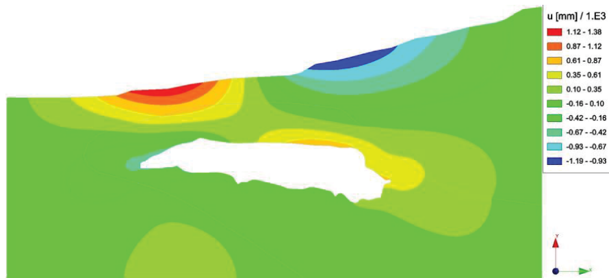
Fig. 8 Horizontal displacements in section 6-6' scalar representation (Option II) – u , in mm
